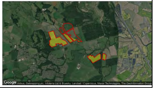
Observer Location Sun azimuth range is 277.1° - 285.1° (yellow)
